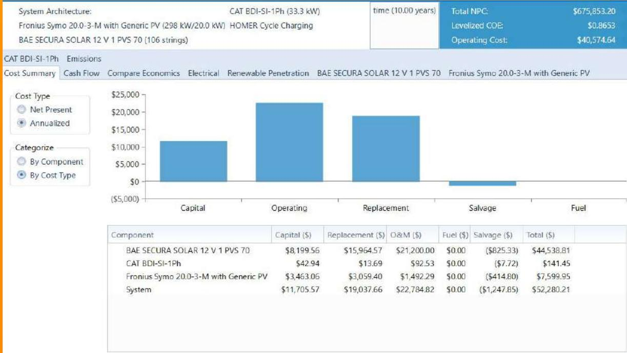
The tool is also capable of optimizing the cost of a hybrid power system (i.e. combination of multiple systems or components), from utility-scale and distributed generation to standalone microgrids.
